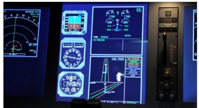
Figure 7: Human-Machine Interface for refuelling manoeuvres in the System Display [21]
